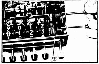
Figure 6-6 Trimming the Right-Hand Wheel.
